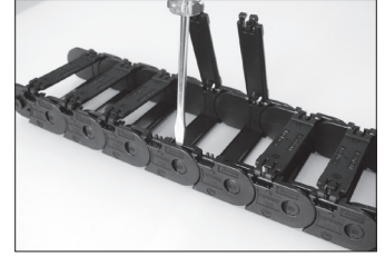
Insert a flathead screwdriver and turn 90° or raise and pry open.
