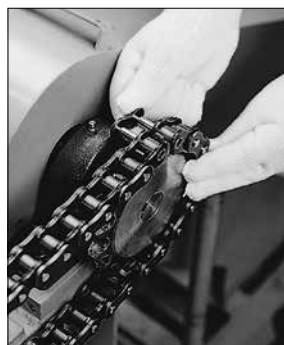
Fig. 8 Connecting on a sprocket
