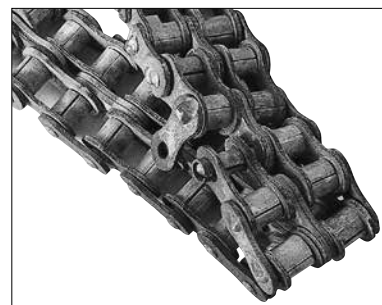
Fig. 34 Corrosion of stainless steel roller chain
