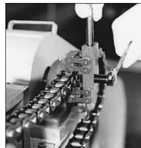
Fig. 5 How to cut a chain using a chain screw1 Rivet-type roller chain
